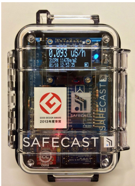
The bGeigie Nano is the current workhorse of Safecast's radiation measurement efforts.
